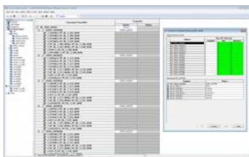
Constraint templates enable application of complex rules to multiple nets
